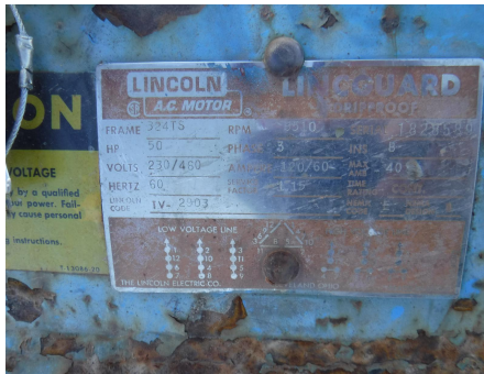
MOTOR ELECTICO LINCOLN MOTORS 324TS, 50 HP, 230/460 VOLTS, - -
